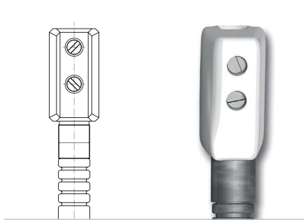
Ceramic terminal connector "plug 'n' heat" Temp. resist. 230 °C / 445 °F Short term max. 280 °C / 535 °F 14 x 21 x 25 mm / 5.51 x 8.27 x 9.84" available with stock items
